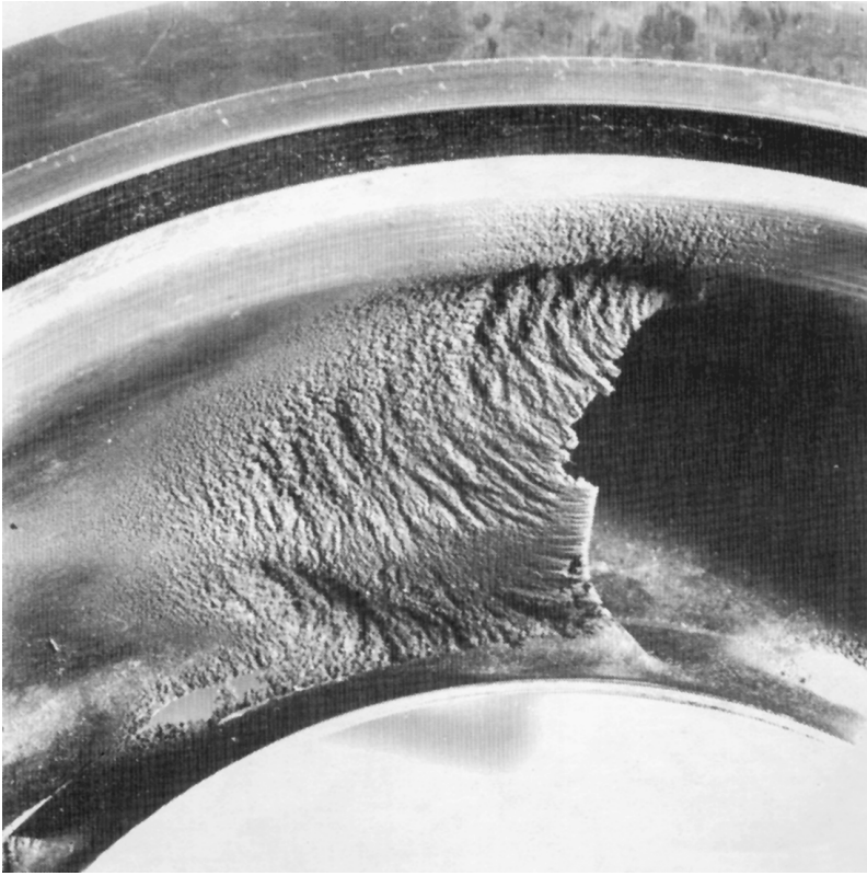
FIGURE 54 Cavitation damage of the impeller blades in the inlet region. 24
