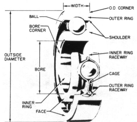
Figure 6.4.4 shows a typical bearing with the various parts identified. Various bearing manufacturers may use slightly different terminology, however, those indicated are the most commonly used.
