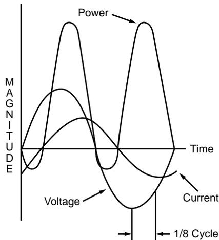
Voltage lags the current by 1/8 cycle or 45 degrees. Power curve showing instantaneous values of power for circuit having equal quantity of resistance and inductive reactance
