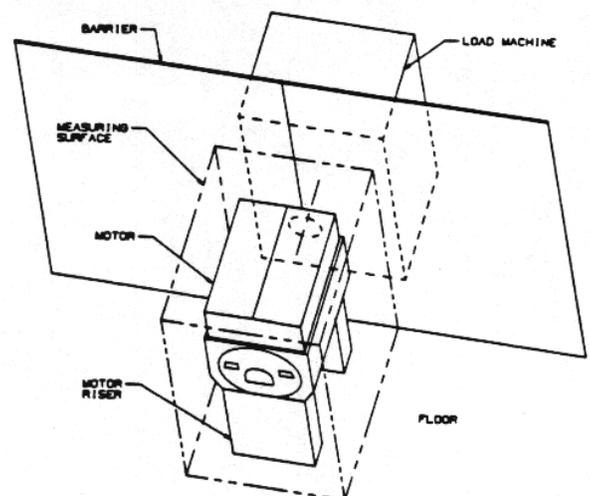
Sound intensity readings are taken at points on each of the four planes of the measuring surface.
