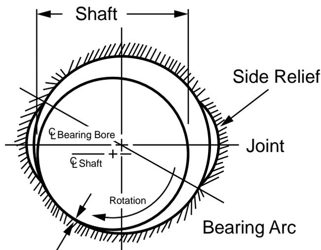
Min. oil film .001" to .005" near this point when operating normally
