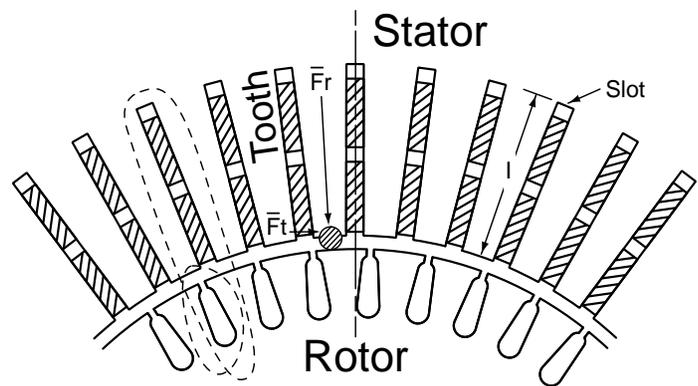
Fig. 5: Magnetic field around rotor bar and resulting forces
