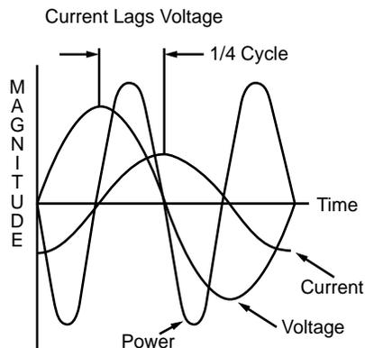
Power curve showing instantaneous values of power for circuit having pure inductive reactance.
