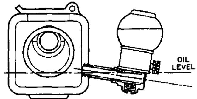
Figure 6.4.25 - Oiler and connecting pipe not level.
