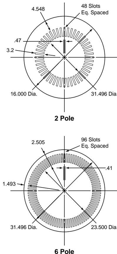
Figure 9: Comparison of two pole and six pole punching
