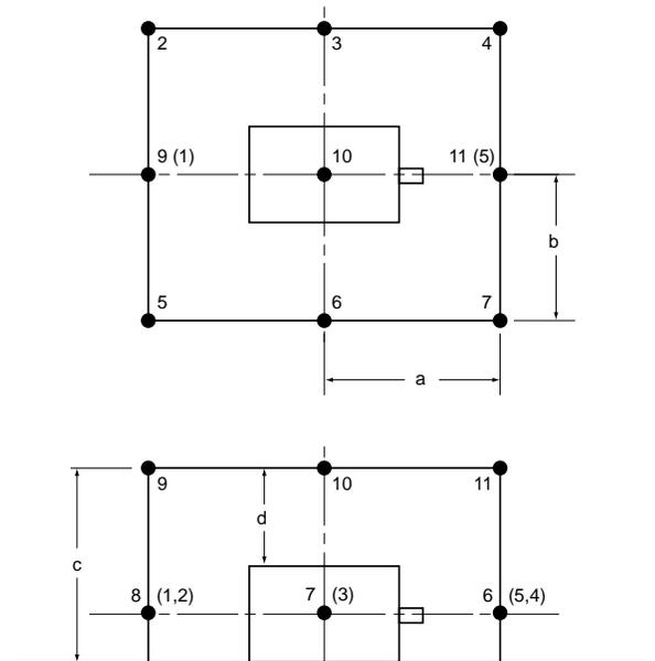
Figure 10: Prescribed Points, Medium Machine (all points of measurement shall be located on the rectilinear planes prescribed, where d is equal to 1 m or greater).
